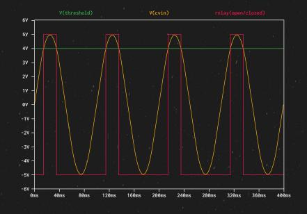
Similarly if we apply a Threshold voltage of -4V we get the inverted relationship of what we saw in the last example.
